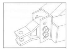
The Hitch is designed to give 3 height positions. The hitch must be set to the proper hitch height to keep the CADDY parallel with the ground.
